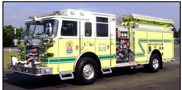
Metropolitan Washington Airports Authority Pierce Pumper on an Arrow XT Chassis
